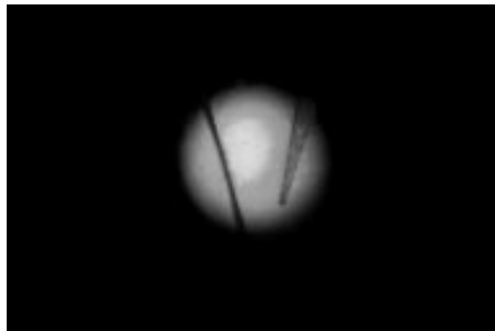
Fig. 2b. Tapered end of dielectric, which forms the transition to metal waveguide; a hair is shown on the left to the same scale.
